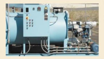
Hybrid Evaporators can be run using natural gas, methane, heating oil or electricity. The boiler provides hot oil to both the heating drum and the rotating rotor.
