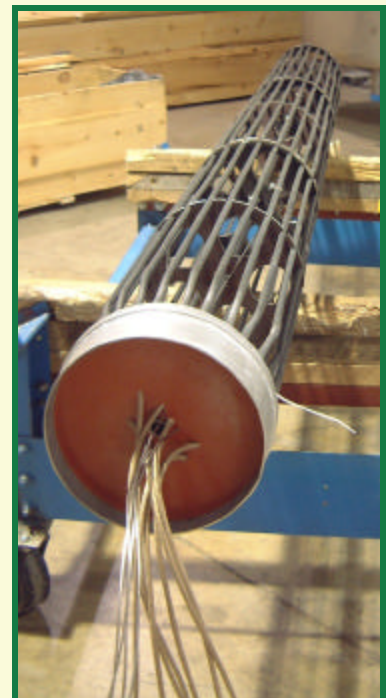
Internal rotor heat tube assembly used to produce Class A Pasteurization
