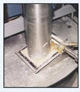
The slaker inlet connector pipe is specially designed to connect the slaker to the lime feeder. The inlet connector design allows the slaker to float on the suspension system without interference from the lime feeder
