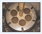
The agitation/mixer system consists of an externally mounted motor located on top of the slaker, a vertical shaft and a specially designed impeller. The high level
