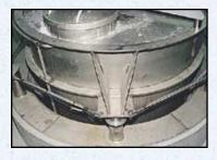
The heart of the RDP Tekkem Slaker is the 3 point suspension/load cell system. The system controls both the slaking process
