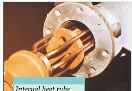
Internal heat tube assembly shown partially removed from the mixing rotor.
