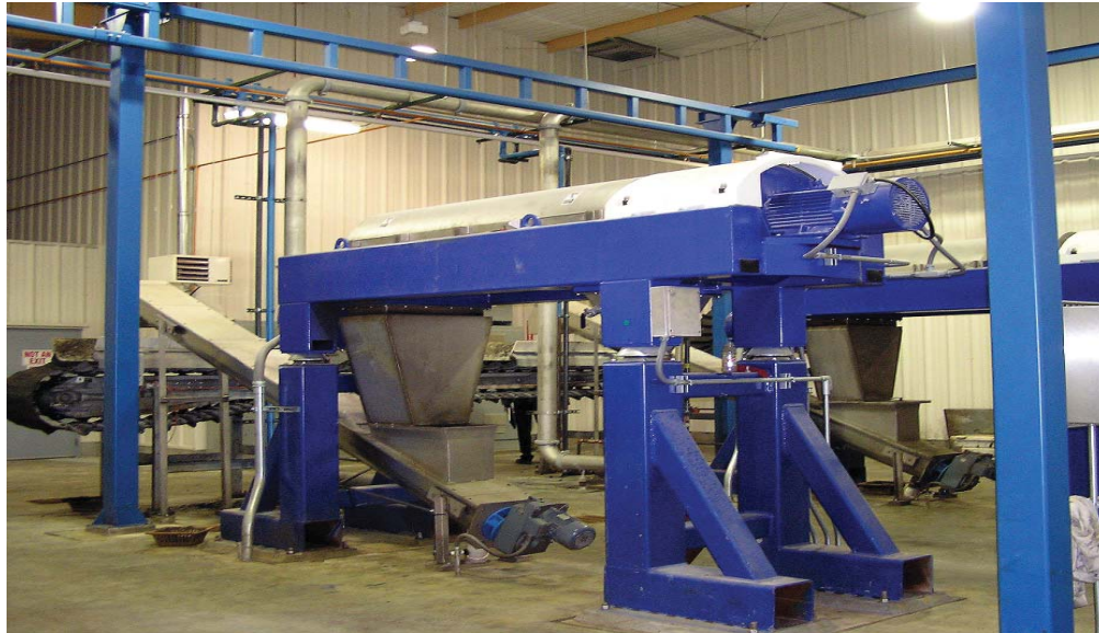
Above: Two centrifuges reliably produce a 22%-24% cake running on 100% WAS.
