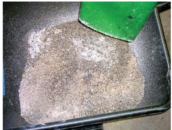
Below: New vibrating screen discharges mainly "clean" grit due to Tekkem's full 10 minutes of slaking time at 185 degrees F.
