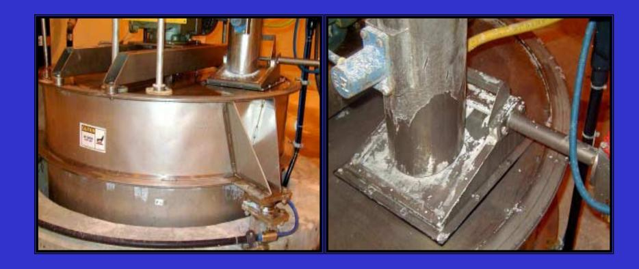
The Slaker sits on 3 load cells and is the heart of the Slaking System. Notice how clean the inlet flapper is due to the Slaker Dust Arrestor.
