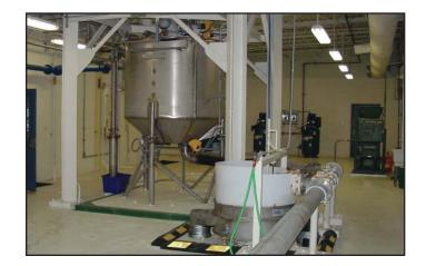
Tekkem Slaker and circular stainless steel vibrating screen
