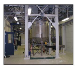
After initial start up of the Tekkem Slakers, the plant reports a quicklime savings of approximately 10%. Further side by side testing of the Tekkem Systems yielded an additional 9% qiucklime savings. The additional savings was achieved by operating the Tekkem Slakers in the Super Heated mode vs the Normal mode. For additional test results contact us at sales@rdptech.com
